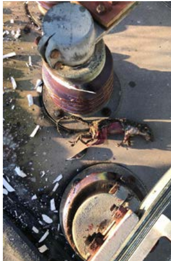
Small mammals such as this squirrel can contact live phases in substations and cause damage to hardware components. Photo credits: Hilton Westman
