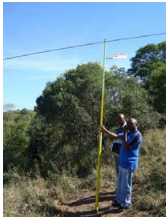
A pole demonstrating the height of the conductor where the elephants were electrocuted. Photo credit: Constant Hoogstad.
