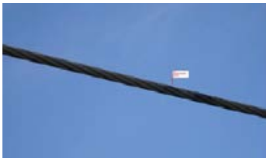
One of the flash marks on the conductor. Photo credit: Constant Hoogstad
